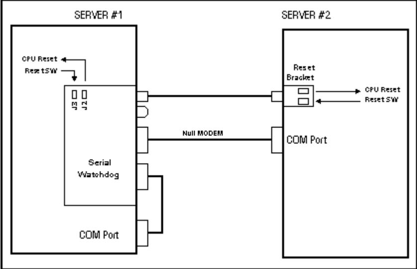
Here we have a master PC with a Watchdog. If it locks up, then its Watchdog card will reset it. If the communications link to the second PC fails as a result of the second PC locking up, then the first PC can reset the second via the external relay and a user program command.
